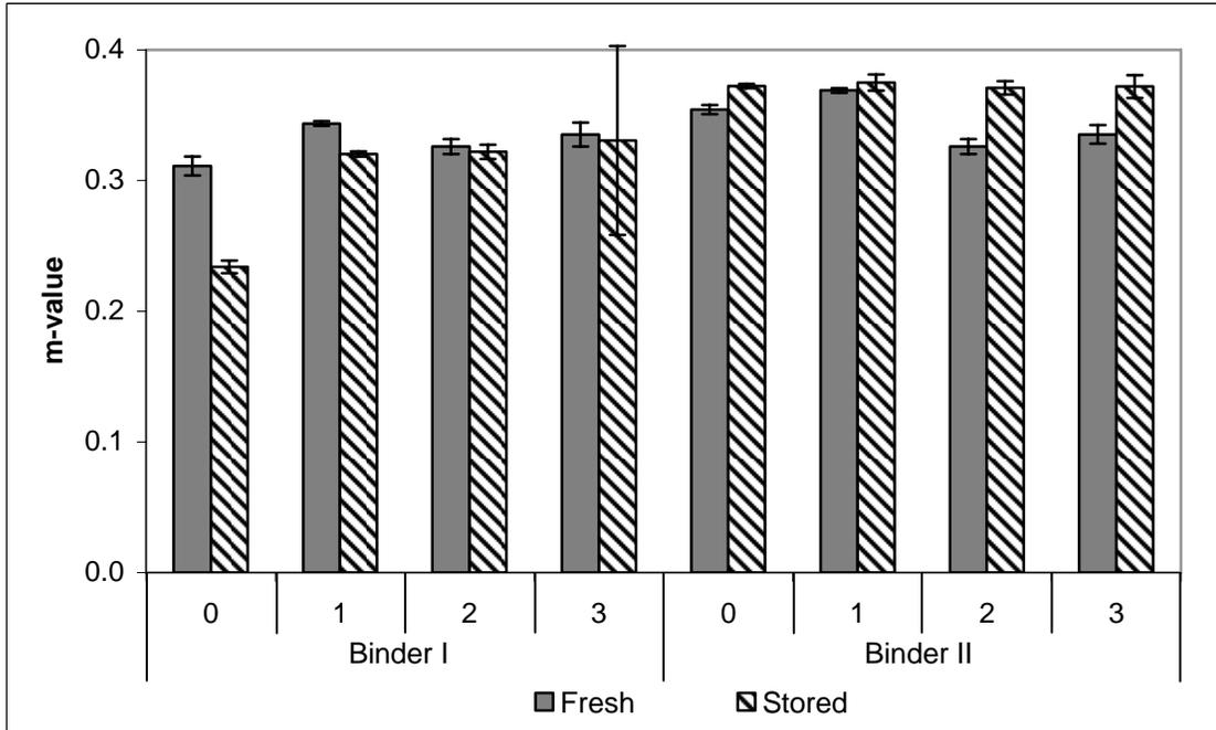
Figure 33: m-value (60 seconds) of fresh and stored binders tested at -12°C.
