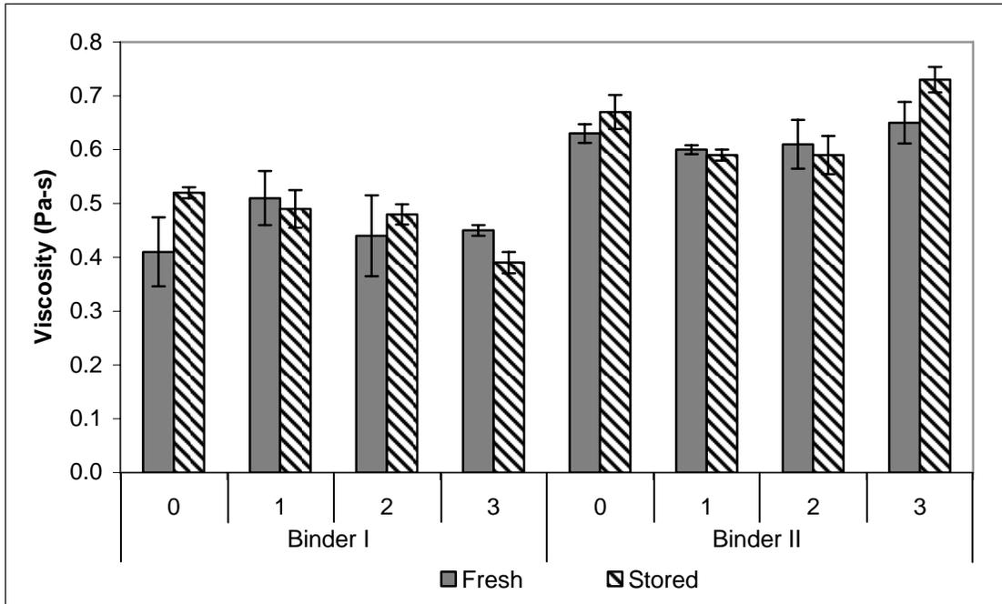
Figure 28 : Viscosity of fresh and stored asphalt binders tested at 135°C.
