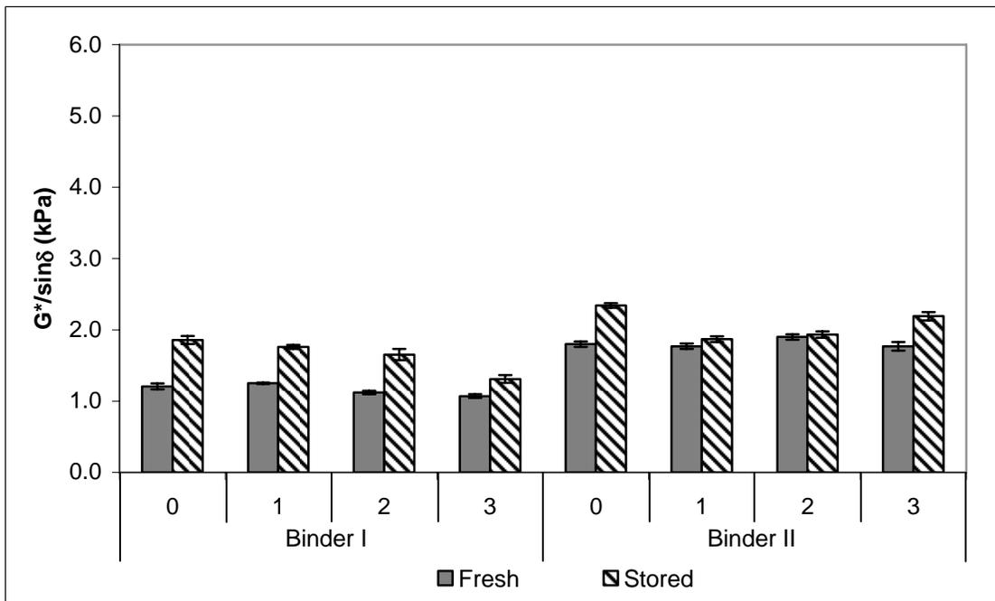
Figure 29 : Original  $G^*/\sin\delta$  of fresh and stored binders tested at 64°C.
