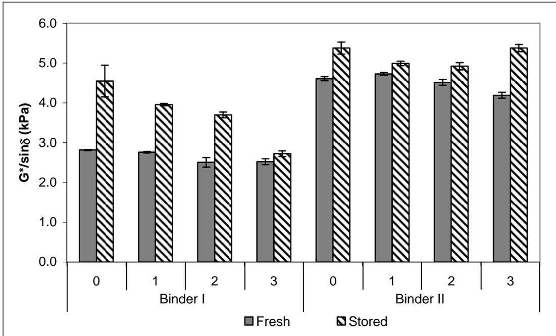
Figure 30:  $G^*/\sin\delta$  of fresh and stored binders tested at 64°C (RTFO residue).
