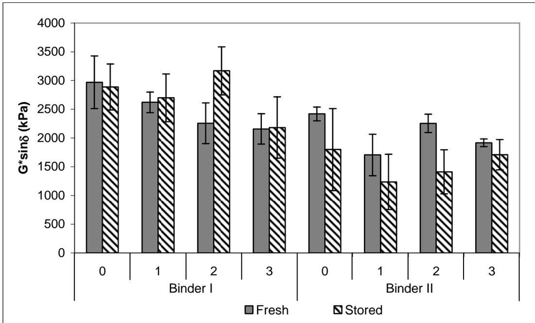
Figure 31:  $G^*\sin\delta$  of fresh and stored binders tested at 25°C (PAV residue).
