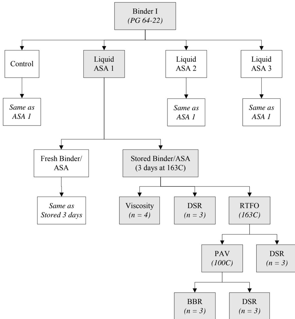
Figure 2: Flowchart for binder testing.
