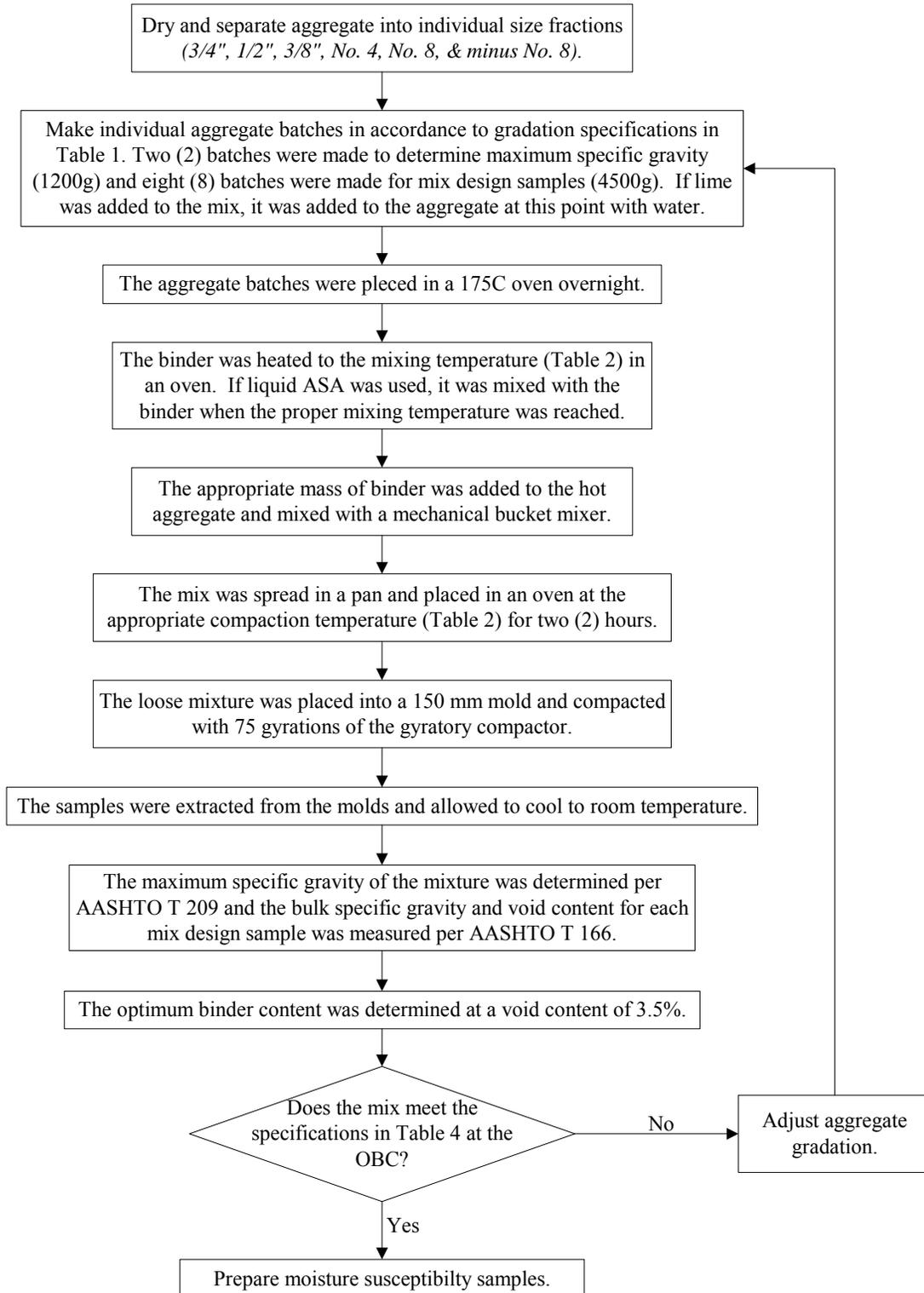
Figure 3: Flowchart of the asphalt mix design procedure.
