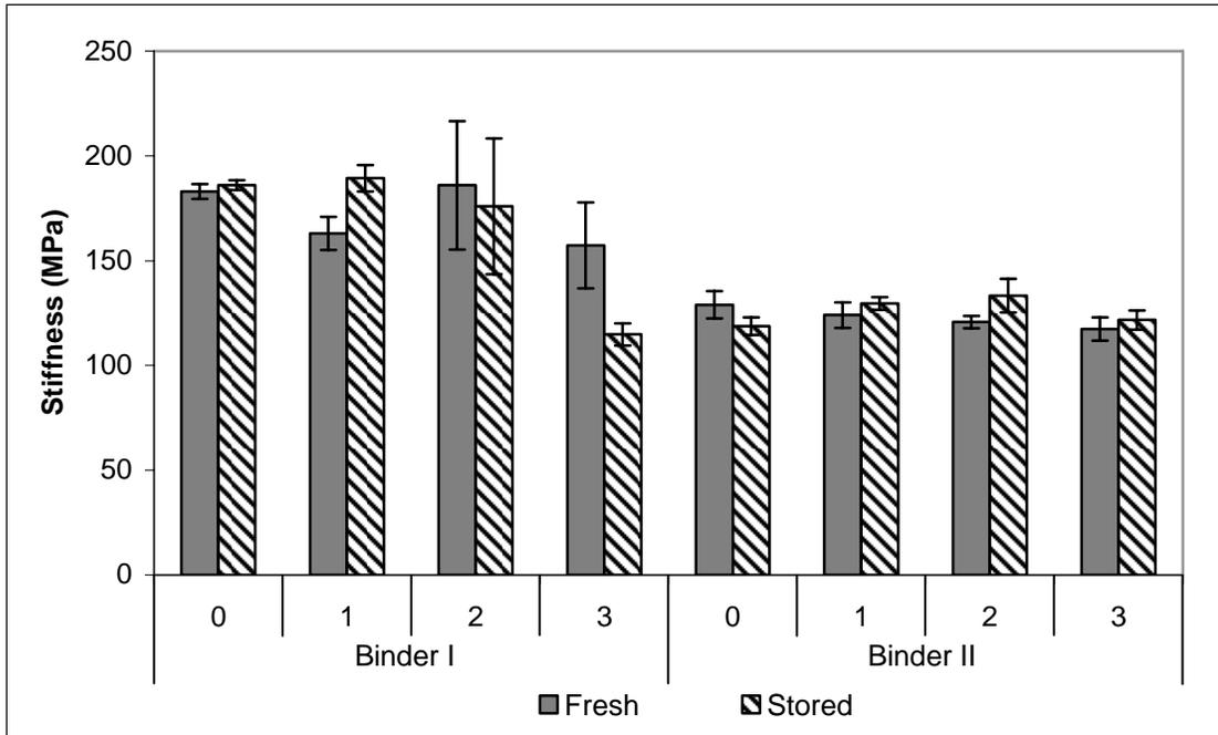
Figure 32: Stiffness (60 seconds) of fresh and stored binders tested at -12°C.
