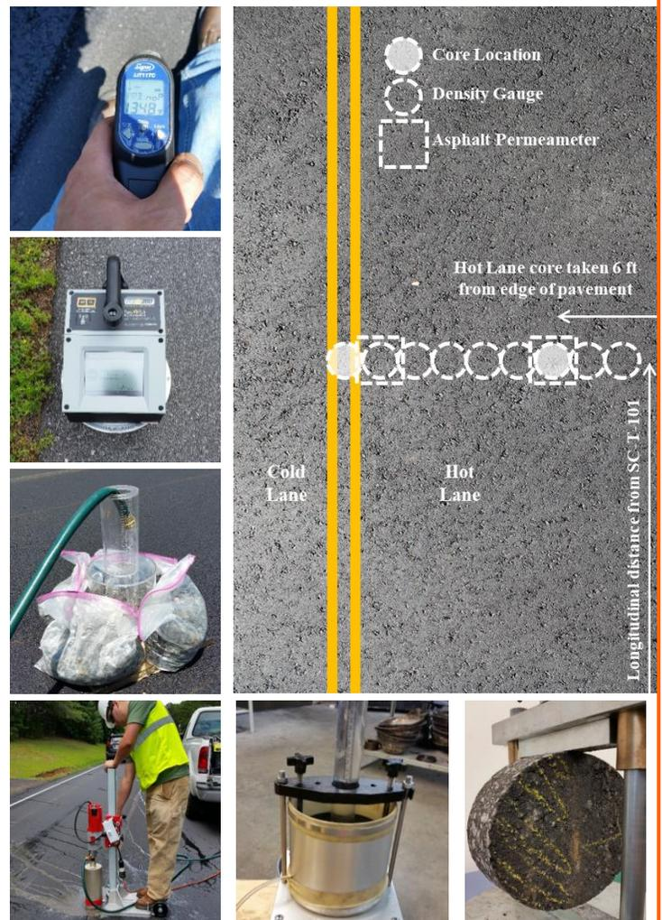
*Longitudinal joint performance was evaluated in the field and cores were taken to assess lab performance.*
