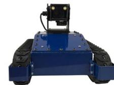
Robot for culvert inspection
